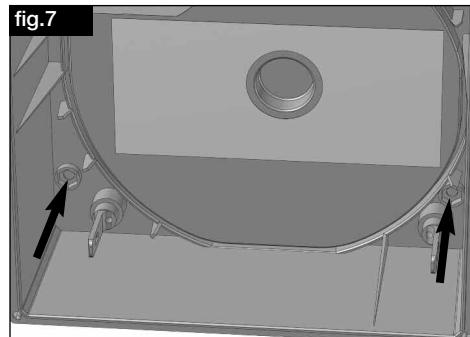
Drill screw adapter for wall fixing
