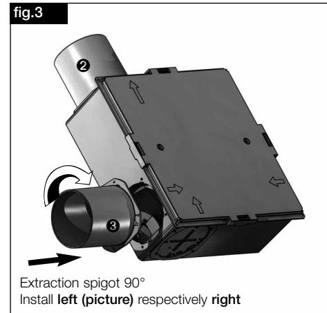
Up to three extraction spigots can be installed (see fig.4).
