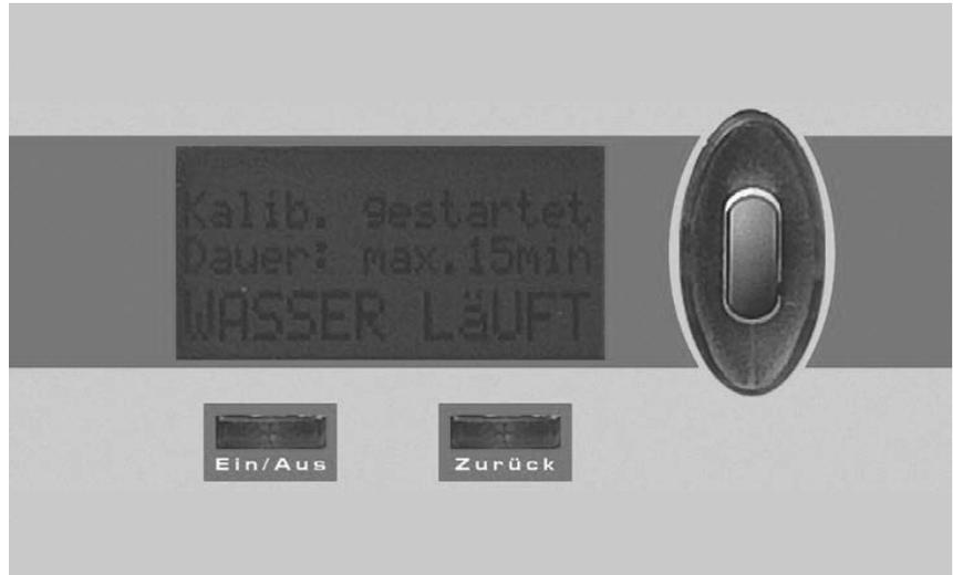
The first two lines on the *display* show the operational menu, the third line shows the operational status.
